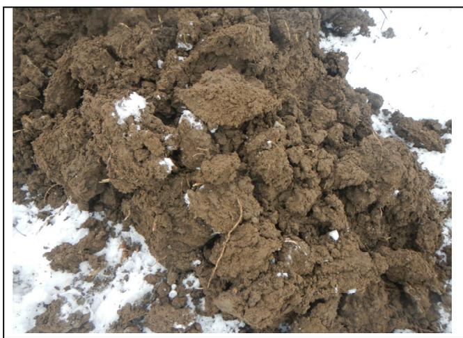
A close-up photograph of dark brown, clumpy soil, likely topsoil, with some snow visible at the bottom left corner.                                                      | <p>Foto 1:</p> <p>BV Flst.-Nrn. 3003+4109, Nonnenweier,<br/>Baggerschurfe am 27.01.2021</p> <p>Dunkelbrauner Oberboden</p>      |
