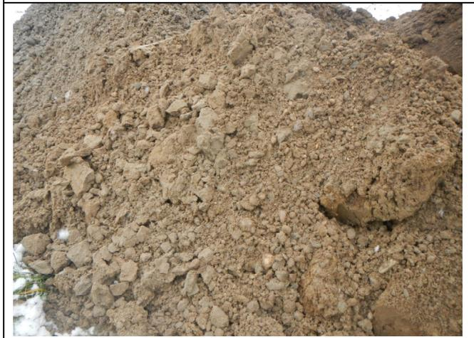
A photograph of a large pile of brown, clumpy soil mixed with numerous small, light-colored stones or gravel, representing a silty sand or siltstone.                  | <p>Foto 3:</p> <p>BV Flst.-Nrn. 3003+4109, Nonnenweier,<br/>Baggerschurfe am 27.01.2021</p> <p>Braune verlehnte Rheinkiese</p>  |
