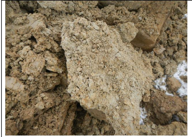
A photograph showing a large, irregularly shaped piece of light brown to greyish-brown soil, possibly a soil core or a large clump, with some snow at the bottom right. | <p>Foto 2:</p> <p>BV Flst.-Nrn. 3003+4109, Nonnenweier,<br/>Baggerschurfe am 27.01.2021</p> <p>Braun bis hellgrauer Auelehm</p> |
