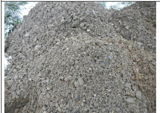
A photograph of a large pile of greyish-brown soil mixed with numerous small, light-colored stones or gravel, representing a silty sand or siltstone.                  | <p>Foto 4:</p> <p>BV Flst.-Nrn. 3003+4109, Nonnenweier,<br/>Baggerschurfe am 27.01.2021</p> <p>Graue Rheinkiese</p>             |
